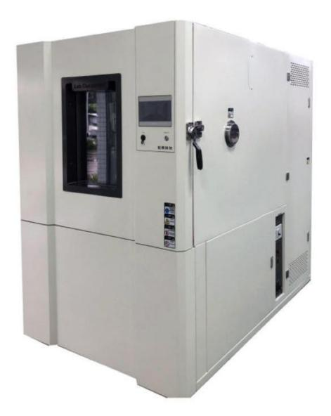
Rapid temperature change test chamber is suitable for instruments, chemistry, plastic, electronics, food, clothing, vehicles, metal, chemical, building materials, aerospace and other parts or machine. With rapid temperature change, gradient adaptability test and temperature stress screening test functions, helps to test the performance and change under the proposed conditions, for the purposes of product design, improvement, identification and factory inspection.
